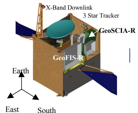
Figure 1 GeoTROPE-R satellite in-orbit configuration.
