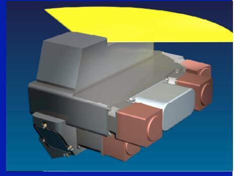
SIFTI (FTIR): O<sub>3</sub>, CO, CH<sub>4</sub>: trop columns and profiles with intelligent pointing for cloud free pixels.
