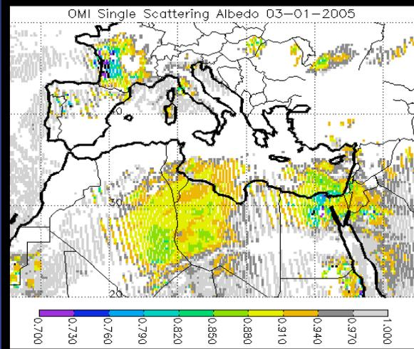
Today: TOMS and OMI take advantage of Rayleigh-aerosol interaction and low surface albedo in the near-UV to retrieve single scattering albedo.
