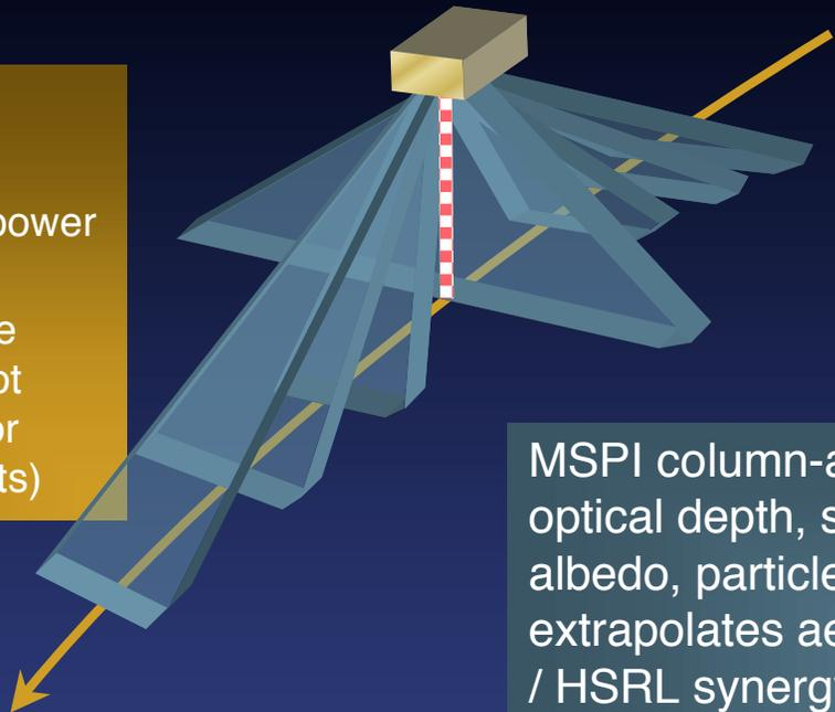
HSRL measures layer-wise profiles of aerosol properties (eff. radius, complex refractive index, shape, concentration), plus column optical depth
