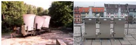
**Fig. 1.** Measurement devices: SODAR for mixing layer height and PM mass concentration sampler.
