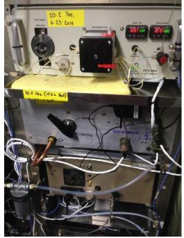
Dynamic blank measurements are taken for 10 minutes at the beginning and end of each flight by passing sample air through a highefficiency particulate air (HEPA) filter. A manual 2-way valve determines the airflow to the filter or sample. The instrument is operated using LabView software to control the auto-collector and sampling time, as well as to monitor and record temperature fluctuations.
