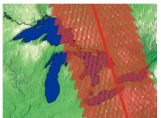
Detection of thermal radiation at 4.7µm for CO, using gascorrelation radiometry
