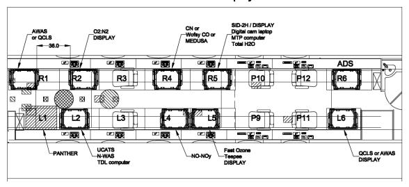
Final payload configuration requires some further discussion about instruments to be placed in Rack 4 (R4). Possible instrument combinations for this rack potentially include 2 of the following 4 instruments (depending on final weight/size/power of all of the instruments on the payload): a) VUV CO (NCAR); b) UV O3 (NOAA); c) Condensation Nuclei (RAF); d) MEDUSA (NCAR). Atlas requested input from the science team on the desired instrument combination for this final rack.
