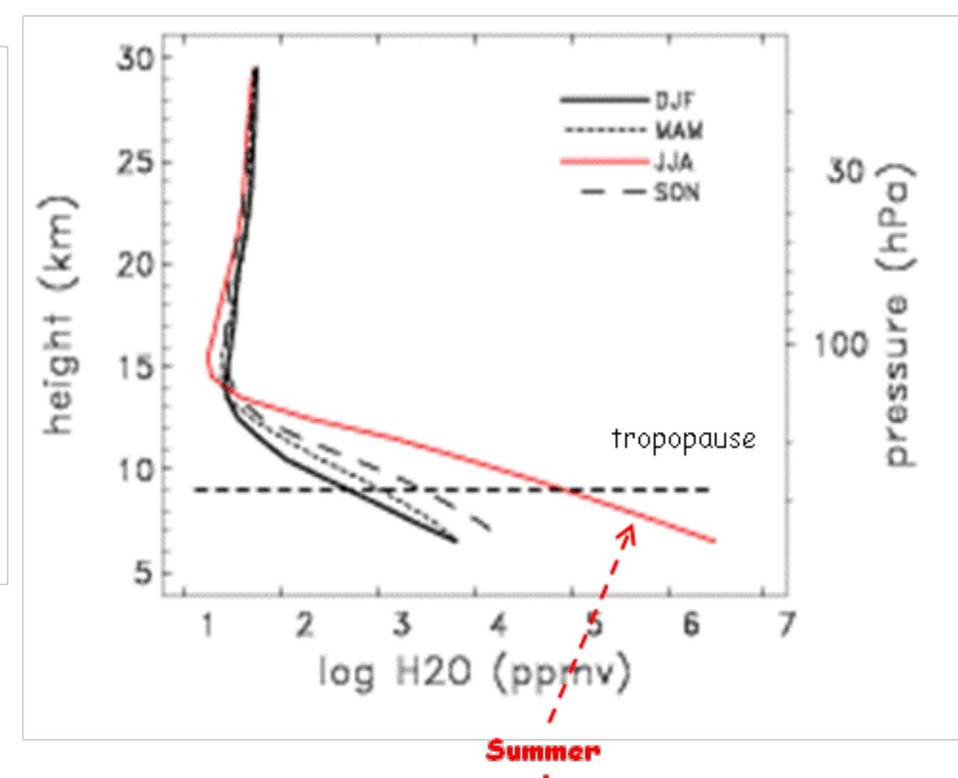
Polar water vapor measurements from the ACE-FTS satellite show a large seasonal cycle, with maximum during summer (an order of magnitude increase compared to winter). This is primarily due to tropospheric temperature variations (the relative humidity is more constant over the year). Note that the water vapor variations extend into the lower stratosphere (the tropopause mixing layer), discussed using ACE-FTS data in Hegglin et al. 2009.
