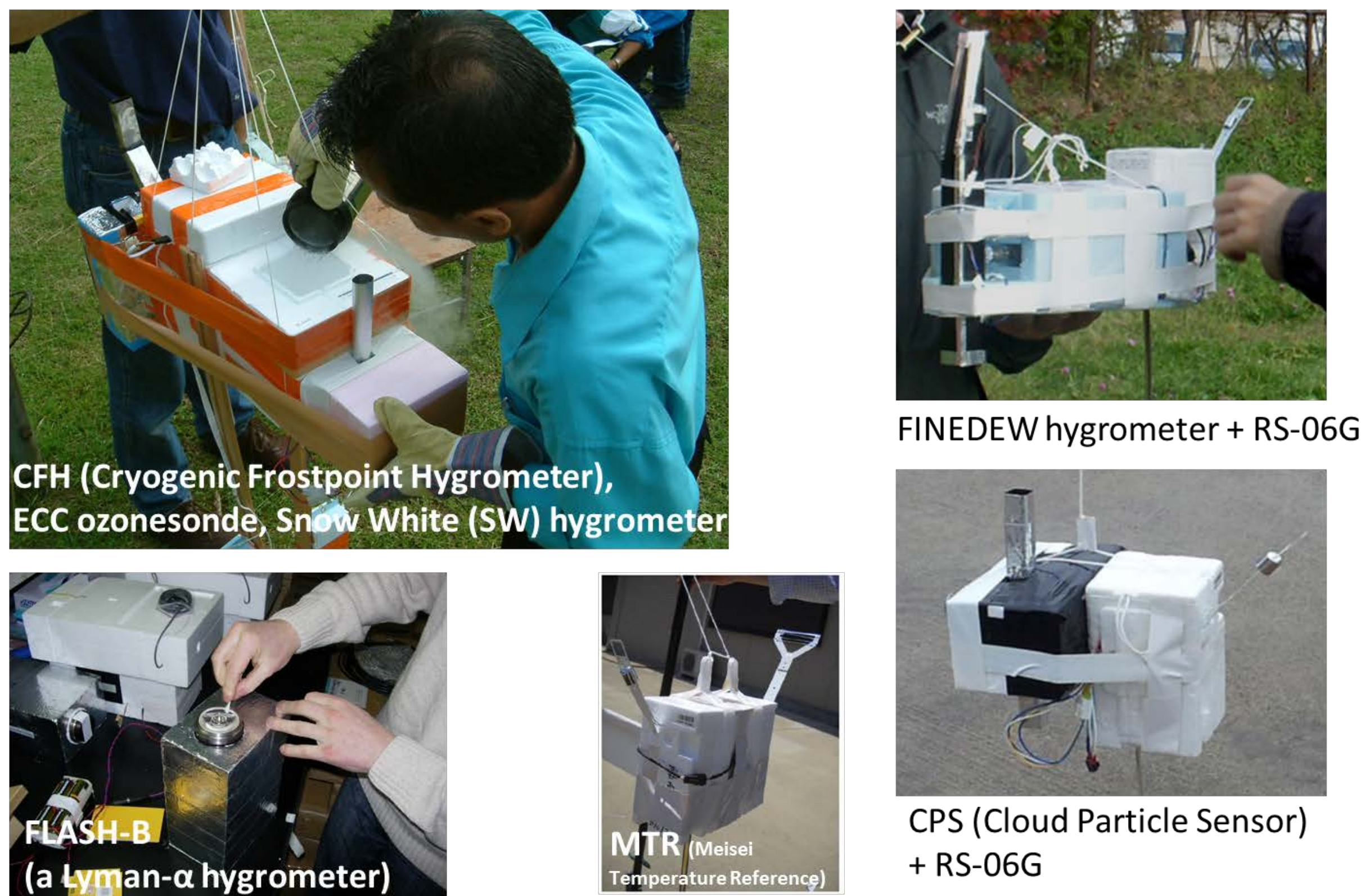
Figure 2: SOWER's main measurement tools: Special sensors on meteorological balloon-borne radiosondes. The lidar systems for particle measurements are also being operated.
