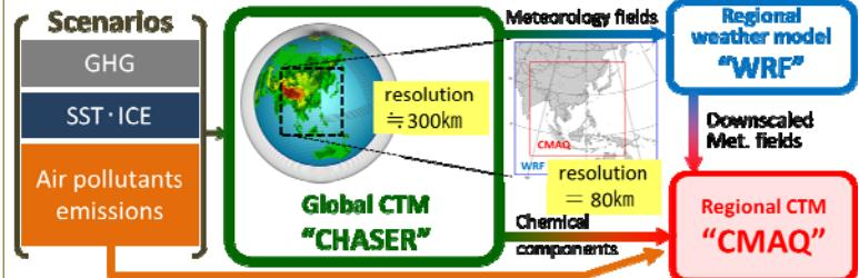
Input scenarios into global CTM to get global meteorology and chemical component fields, which are then downscaled with WRF/CAMQ system.
