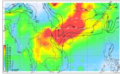
Figure 2. Maps of (a) 0.5°x0.5° gridded total fire counts, and (b) 1°x1° aerosol optical depth (shaded) and cloud optical depth (contour) at wavelength 550 nm obtained from the MODIS instrument aboard the Terra satellite during March 1 and April 15 2014. The 1°x1° NCEP reanalysis 925 hPa and 700 hPa winds (vector) are also shown in the figure.
