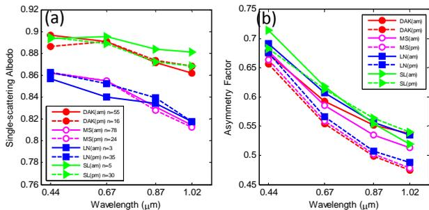
Figure 6. AERONET retrieval of aerosol optical properties, (a) single-scattering albedo, and (b) asymmetry factor as change with wavelength obtained from four sites over northern Indochina during March 1 and April 15, 2014.
