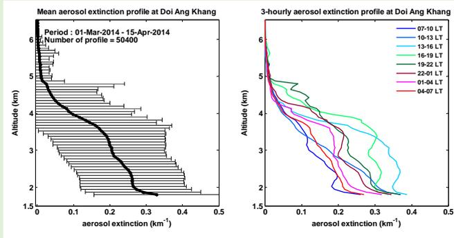
Figure 4. (a) mean aerosol extinction profile with stand deviation and (b) mean 3-hr aerosol extinction profiles in local time during March 1 and April 15, 2014.
