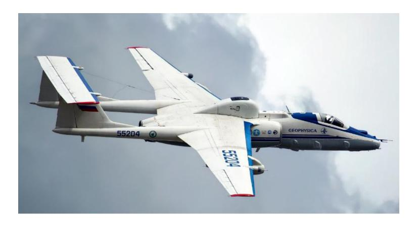
Max. Altitude: ~20km Range: 3500km Max. Payload Weight: 2,000kg Wing Span: 37.46m
