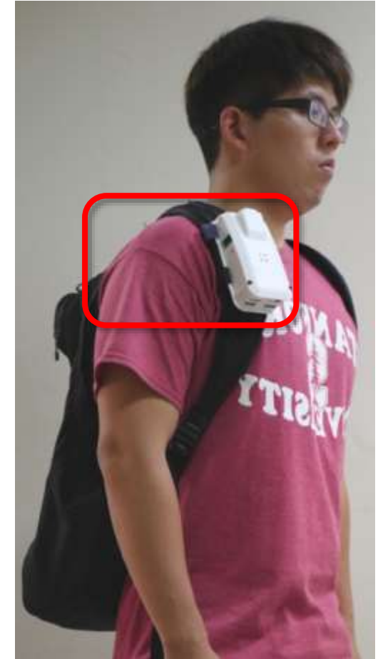
Year of 2017 Wearable PM sensor. Less than 200g with GPS and wifi
