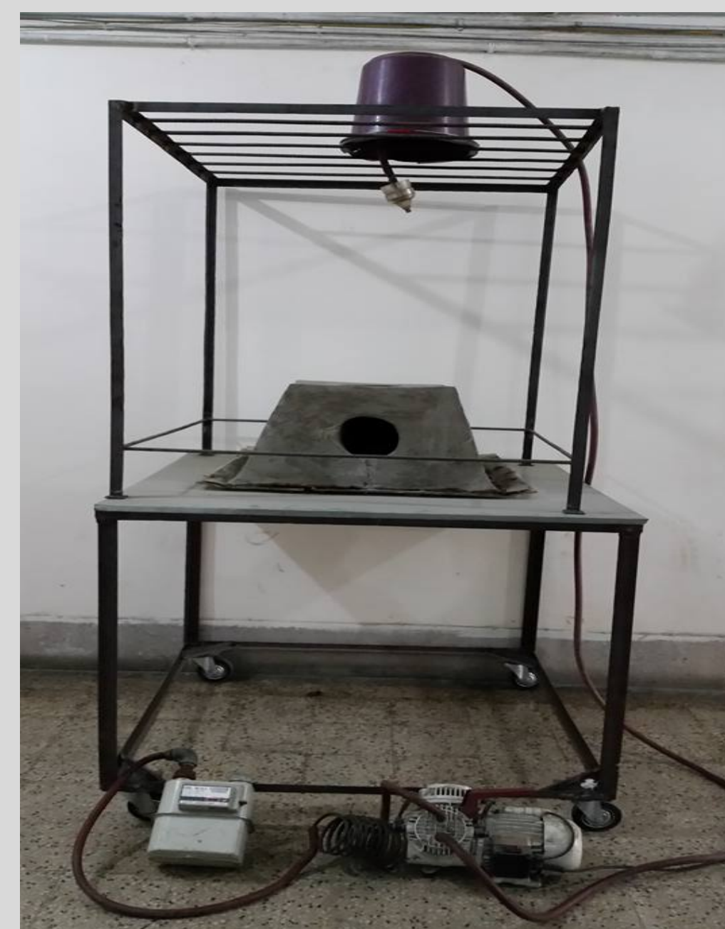
Fig-1: Experimental set up for burning of biomass species
